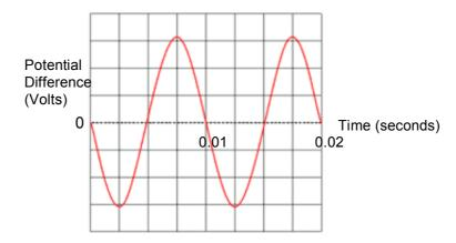
1 (a) (ii) Use the graph to determine the period of oscillation for the supply.
